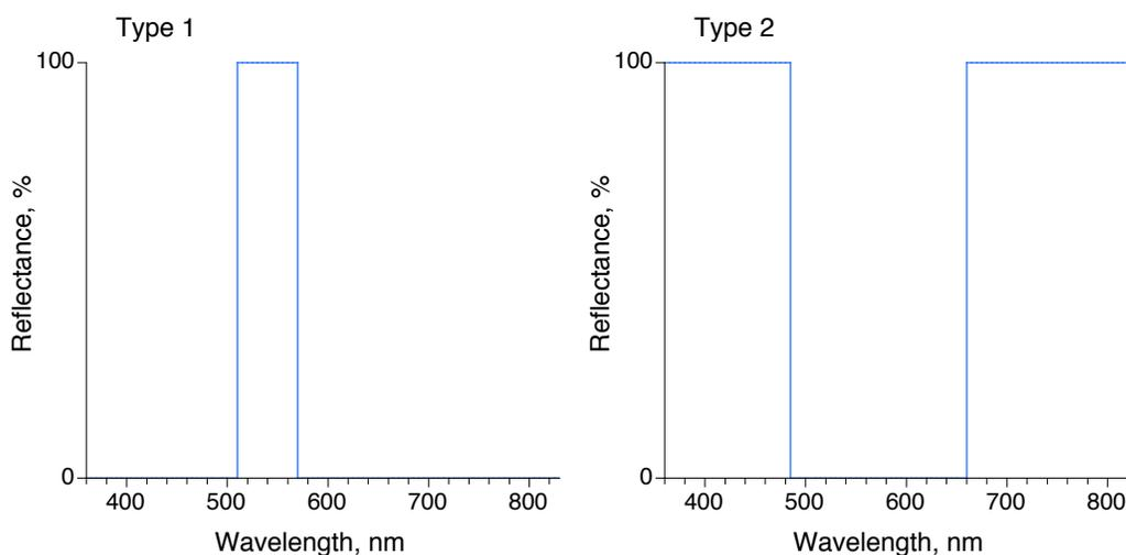
Fig. 1. Examples of the two spectral reflectance patterns of optimal colors. Left: Type1; Right: Type 2
