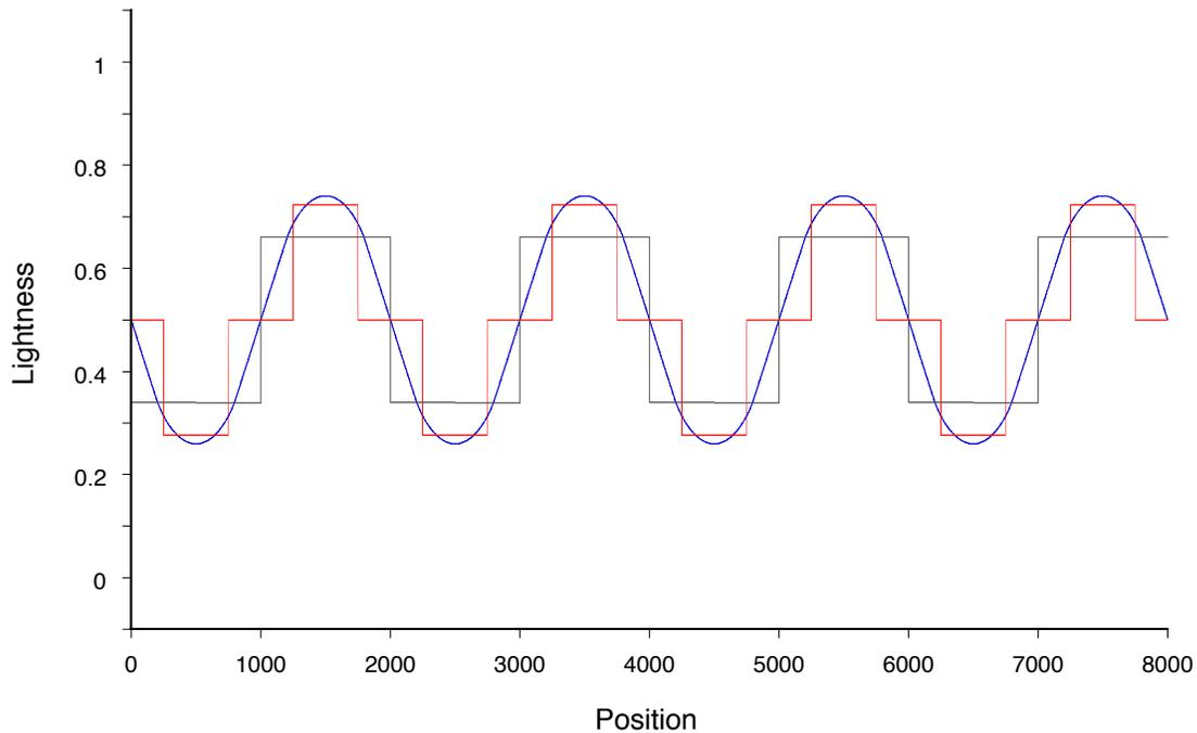
Fig. 3. Lightness values of a grid of photosites superimposed on the blurred lens image of a sequence of four line-pairs. The sampling frequency is four photosites per line-pair. Blue curve: lens image. Red line: photosite lightness values for the maximum contrast photosite alignment. Gray line: photosite lightness values for the minimum contrast case.
