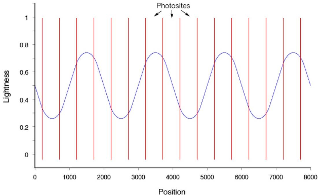
Fig. 2. The blurred line-pair pattern of Fig. 1 with superimposed photosite sampling indicated by vertical red lines. See text for additional explanation.
