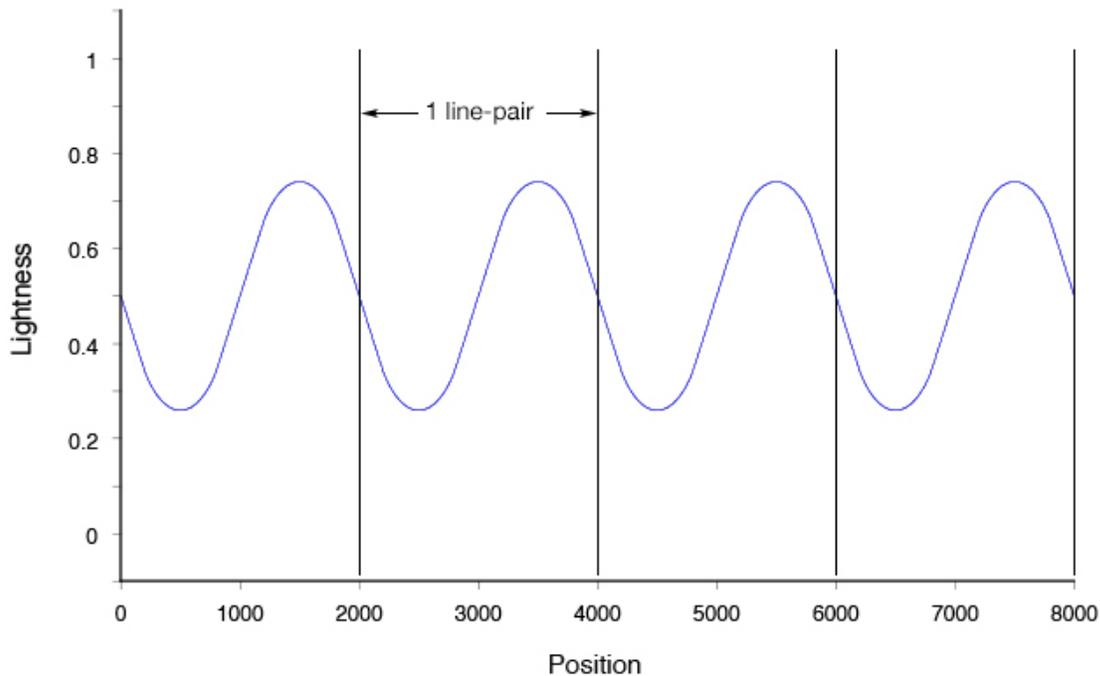
Fig. 1. Representation of a line-pair pattern simulated with a diffraction blur diameter equal to 80% of the line-pair width. Contrast ratio is 48%. See text for additional explanation. Units on horizontal axis are dimensionless.
